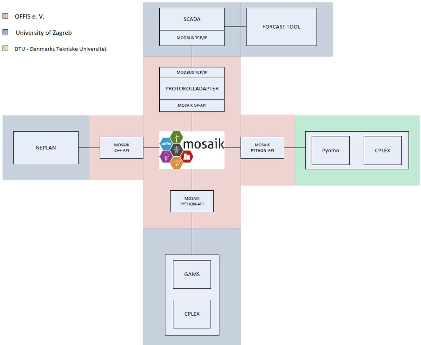
**Figure 4: Overall architecture of the  $\mu$ Grip simulation**
